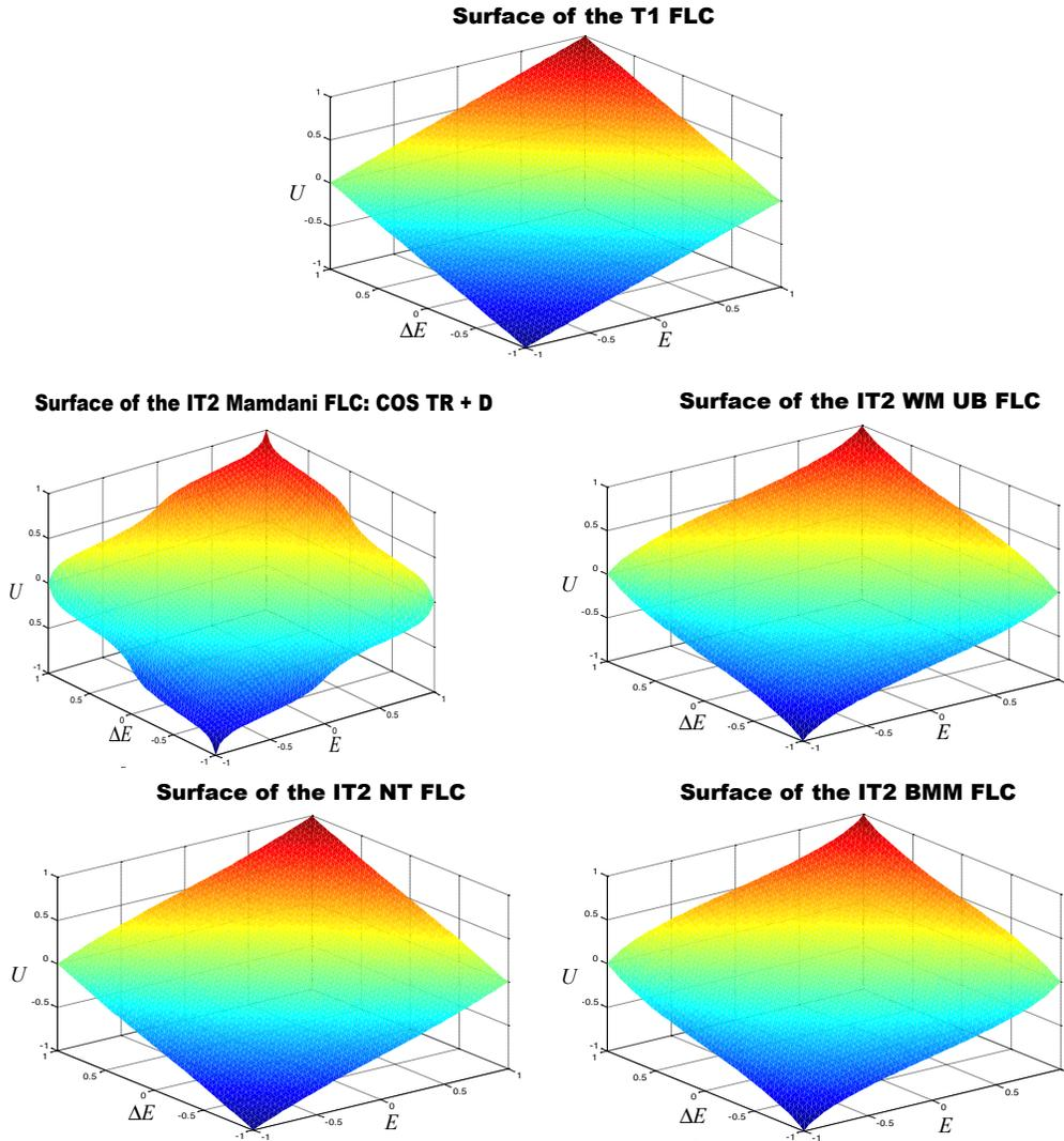
**Figure SM-1:** Control surfaces for T1 FLC and the four IT2 FLCs (Mendel, 2017 [37, p. 606]; © 2017, Springer). “D” denotes defuzzification. The figures were generated, most graciously, by Prof. Tufan Kumbasar.
