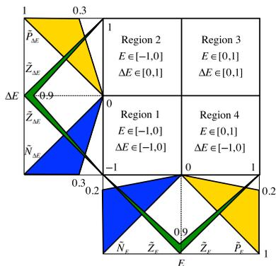
Fig. 8. IT2 first-order rule partitions for the IT2 FPID controller.
